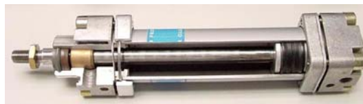
(b) Cross section of a double acting cylinder
