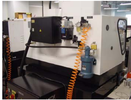
(b) Pneumatic system of an automatic machine
