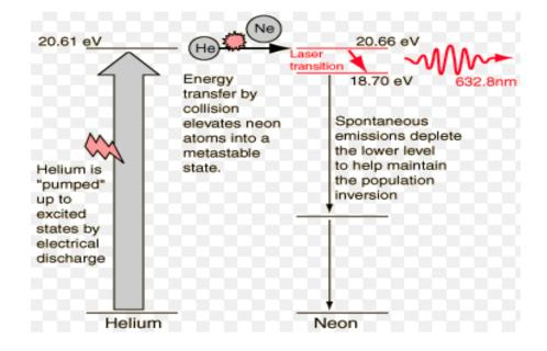
This process is given by the reaction equation:
