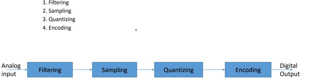
**Filtering :** This **filter** eliminates the high frequency components present in the input analog signal which is greater than the highest frequency of the message signal, to avoid aliasing of the message signal
