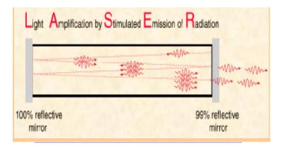
The principle behind such amplification is simple. One incident photon strikes the excited atom in the higher energy state under population inversion condition to produce two photons. If those two photons are reflected back from a mirror and simultaneously, strike another two atoms, four photons have been emitted which are coherent in nature and are in same phase. This process continues for a no of repeated reflections that results the amplification of stimulated light intensity constructively.
